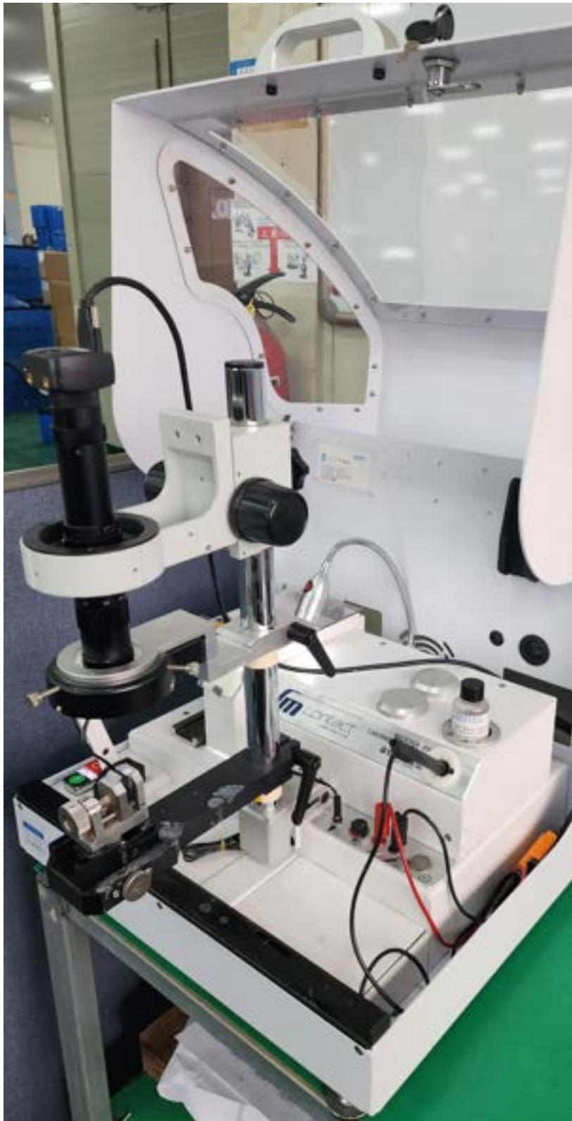
Cross section camera for crimped terminal
